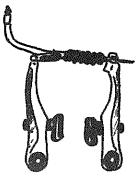
In the last few years, mountain bikes have been coming with V-Brakes (or linear cantilevers) as standard equipment. The brake arm, or 'lever' of a linear cantilever is longer, giving the rider a bit of a mechanical advantage. Another difference is the brake pad, it is much longer so it gives more pad contact on the rim. Some of the more expensive V-Brakes use a parallelogram design for the pad. This parallelogram gives the pad a smooth inward travel as opposed to a curved path of travel.
