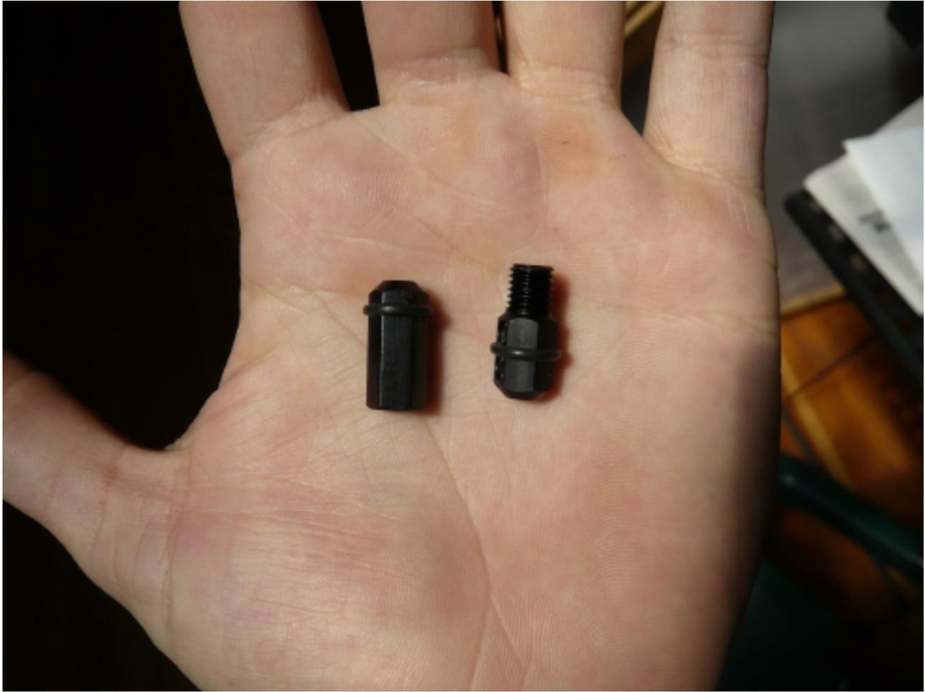
Figure 7: The two halves of a cable splitter.
