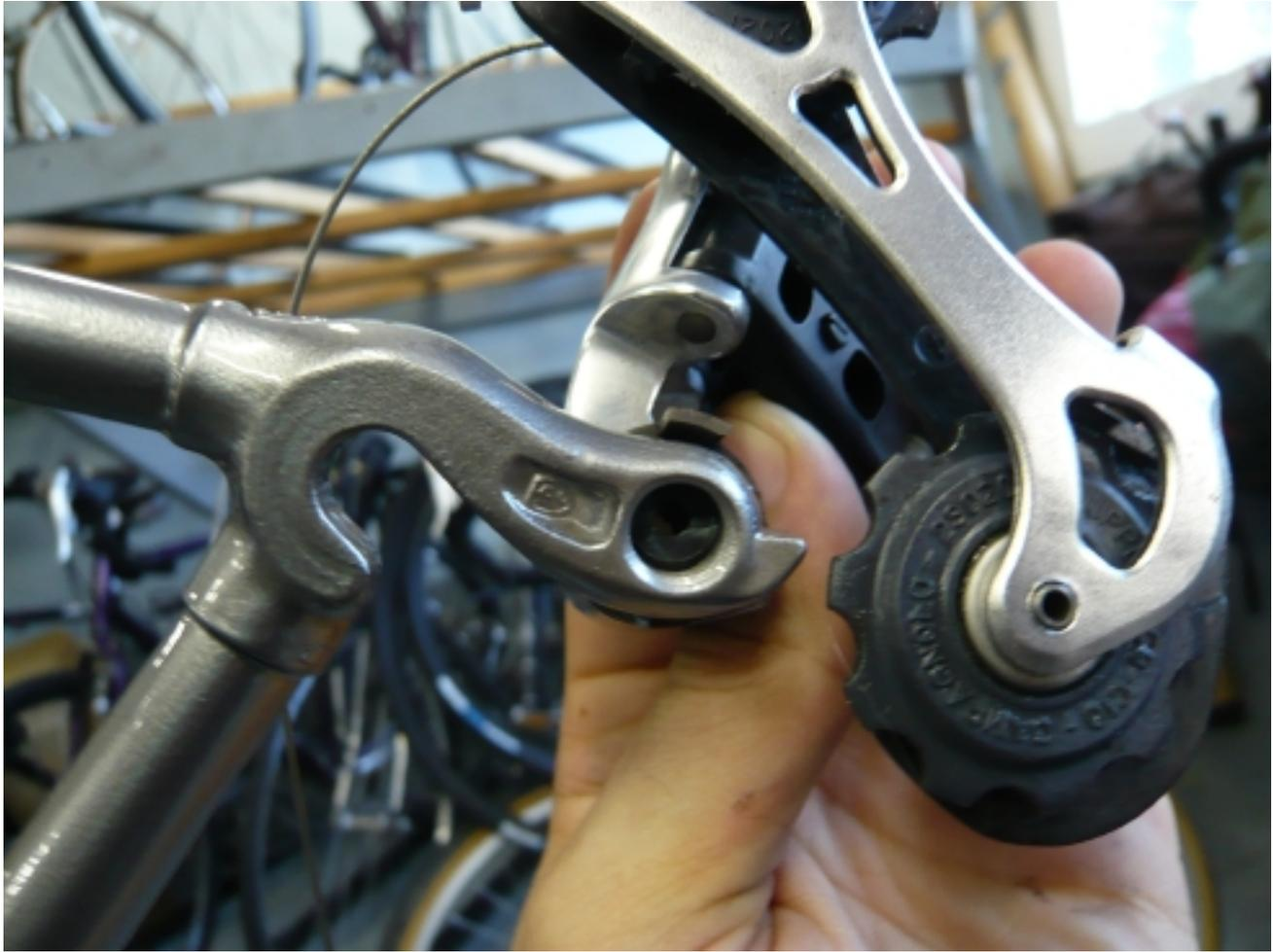
Figure 6: The proper alignment of the hanger and derailleur tabs.
