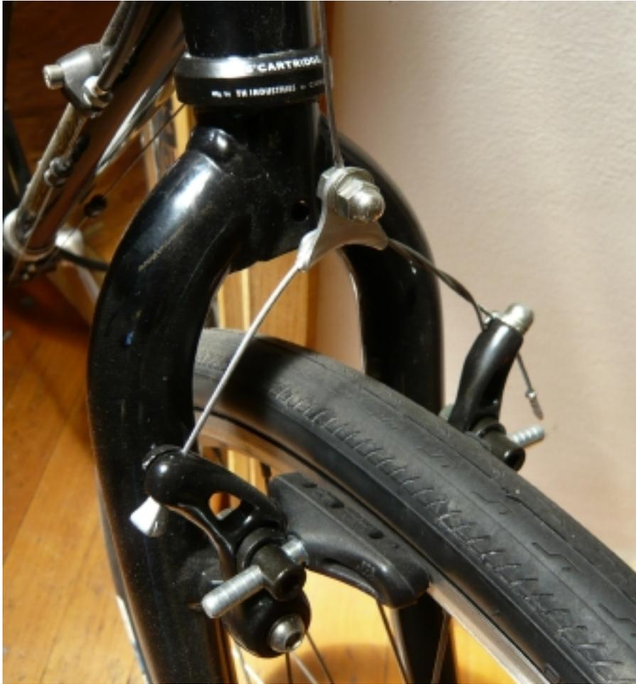
Figure 10: A correctly set up front brake.
