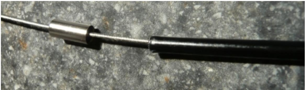
Figure 9: Incorrect: the ferrule is loose on the cable. Avoid this by snugging the ferrule onto the end of the housing.
