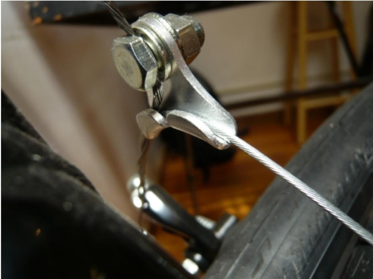
Figure 11: A close-up of the straddle saddle from behind; notice the straddle cable passing through the “hook” of the saddle, and the spare cable wrapping down one side.
