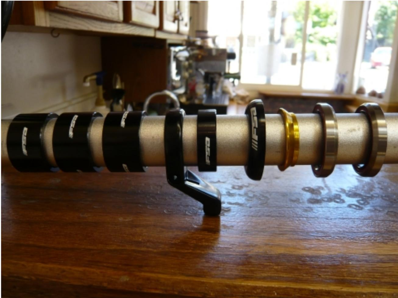
Figure 15: The steer tube stacked with head set parts. From left to right: a number of headset spacers, a cable hangar, another spacer, a head set top-cap, a gold split ring race, and two bearings, beveled edges facing one another.
