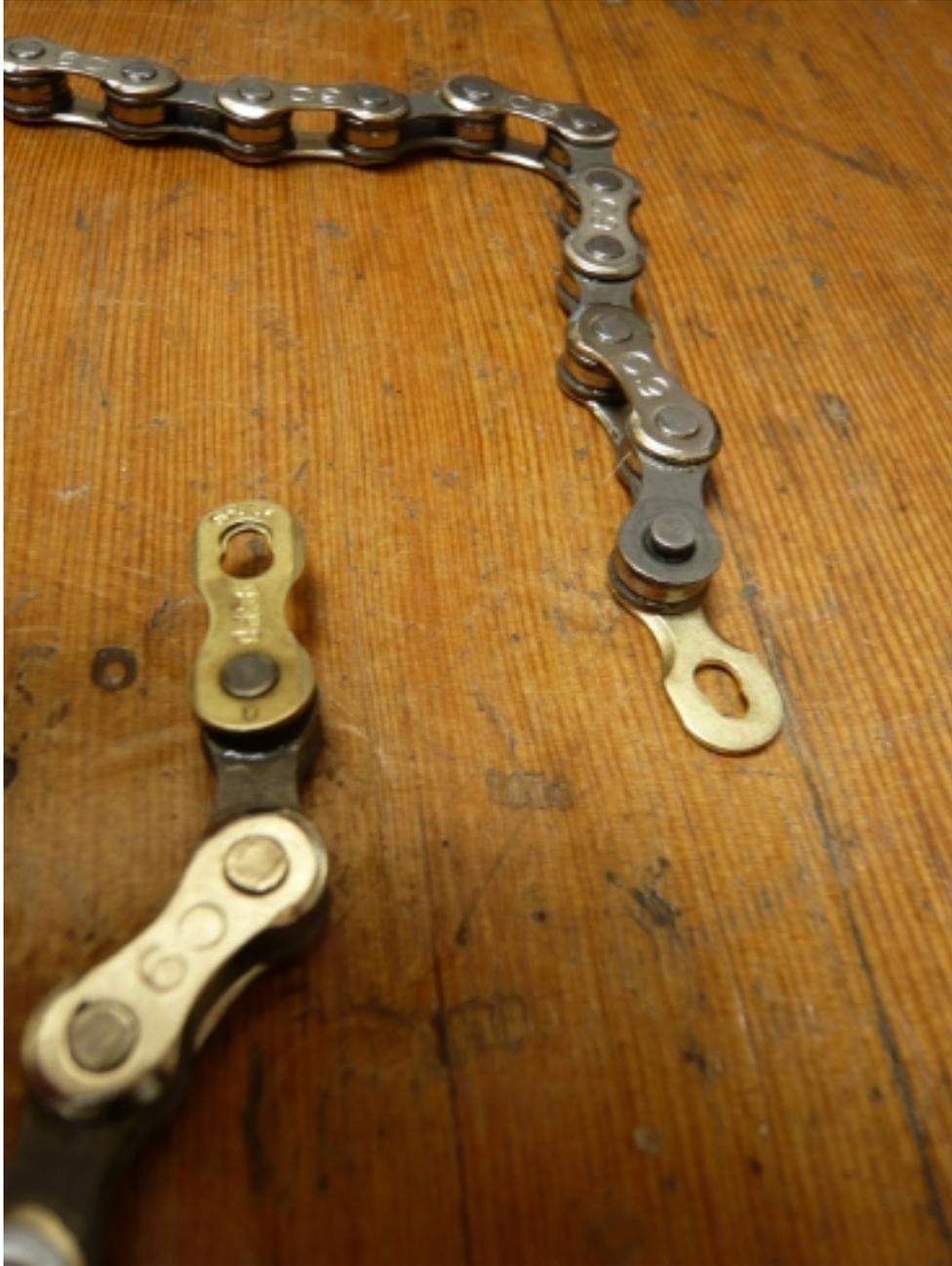
Figure 12: A master link, with each half placed in opposing sides of the chain.
