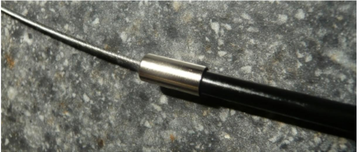
Figure 8: Correct placement of the silver ferrule on the end of the cable housing.
