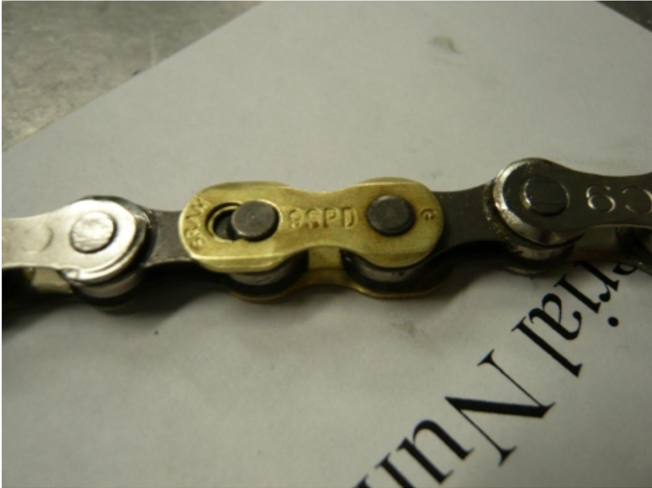
Figure 13: A master link being assembled; the opposite side of the chain would look identical to this picture. From here, the chain need only be pulled and the link will be fully installed.
