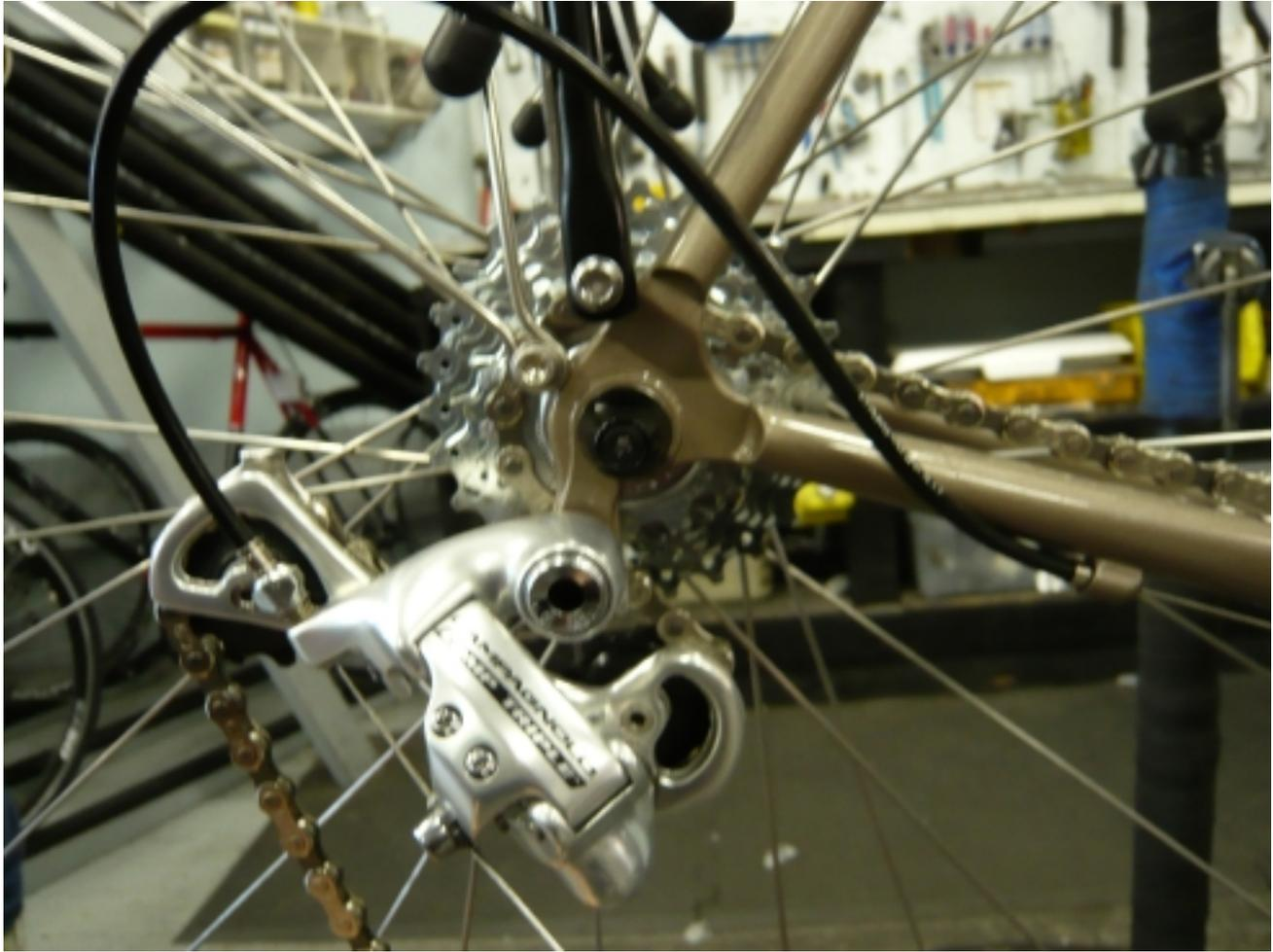
Figure 18: The chain wrapped properly around the cassette.
