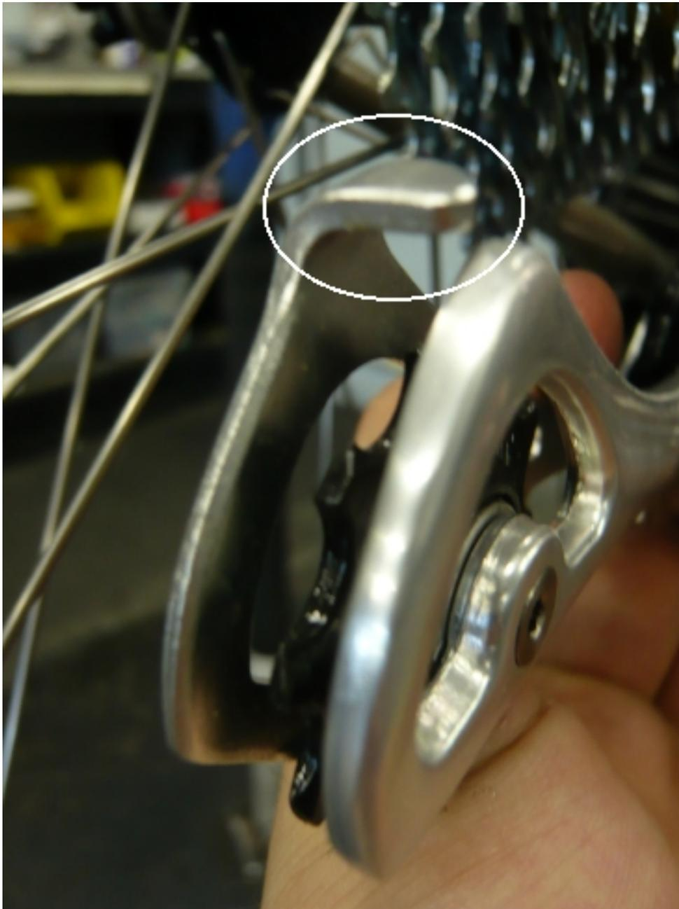
Figure 14: A closeup of the rear derailleur cage, showing the jockey pulley (the black cog) and the metal tab. Each pulley has one of these tabs; make sure the chain routes between the tab and the pulley.
