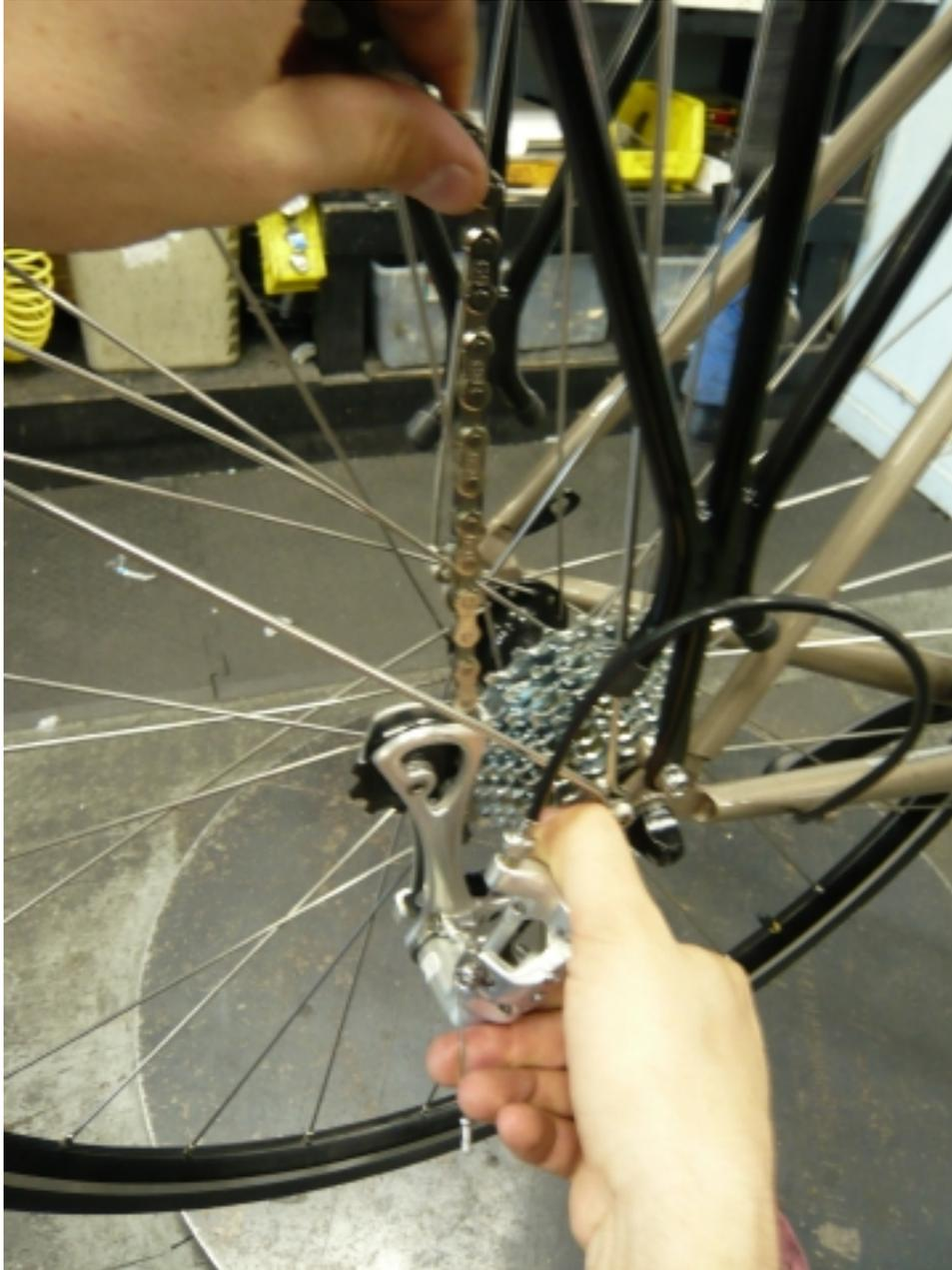
Figure 17: The easiest way to route the chain through the rear derailleur cage.
