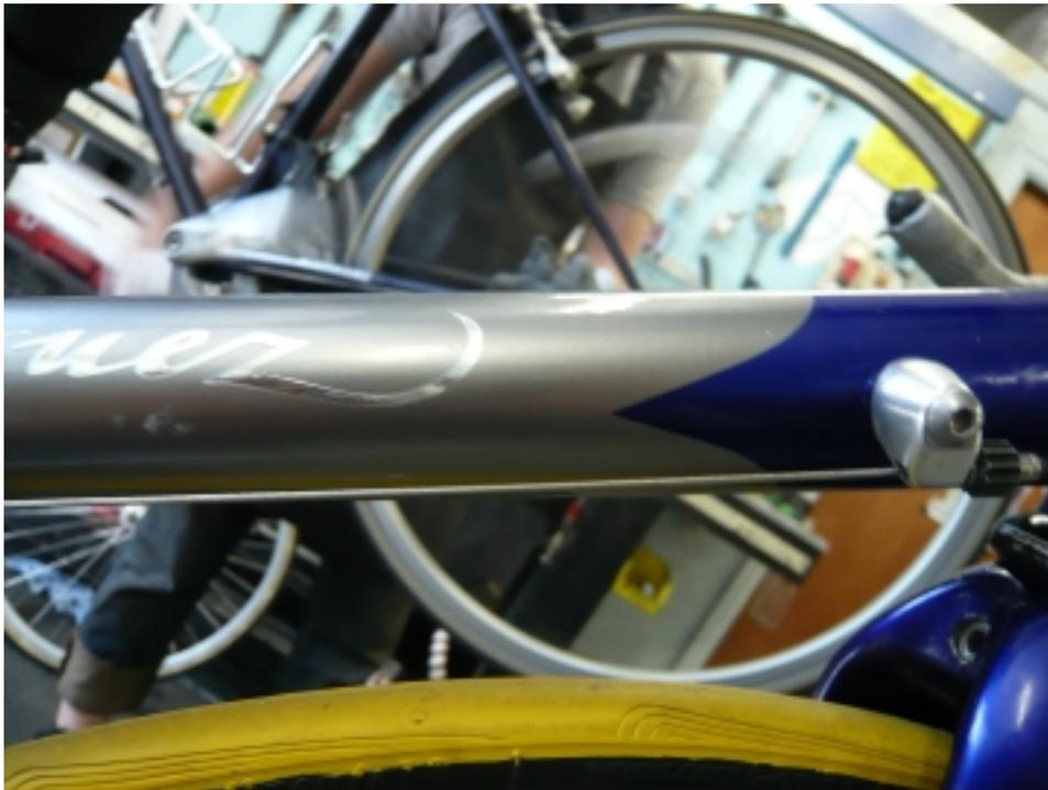
Figure 3: A down tube cable stop, properly aligned. Notice the Rodriguez logo on the down tube; use it to get you relative positioning correct.
