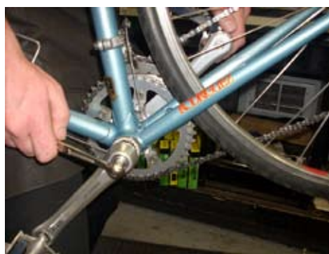
Jeremy having way too much fun installing a new bottom bracket into a 25 year old Rodriguez bicycle. This bike looks great, and was back on the road a day or 2 after the customer brought it in for service. Thanks to the ISO commission of the 1970's, this bicycle will probably be on the road another 50 years or more.
