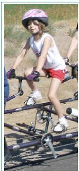
Way back in the late 1970's we used to make something we called the Rodriguez Kidback. It consisted of a kit that allowed you to put a set of cranks up on the seat tube of a tandem to allow for a small child to ride in the stoker position.
